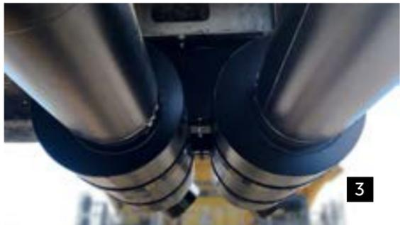
ABOVE Liebherr T282C dual-wall exhaust system, engine pipe and mounting details. Thermal blankets installed on turbos.
