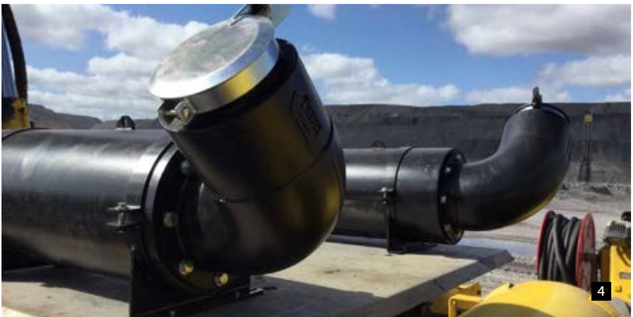
ABOVE Atlas Copco PV275 dual-wall exhaust system, muffler, engine pipe and mounting details.
