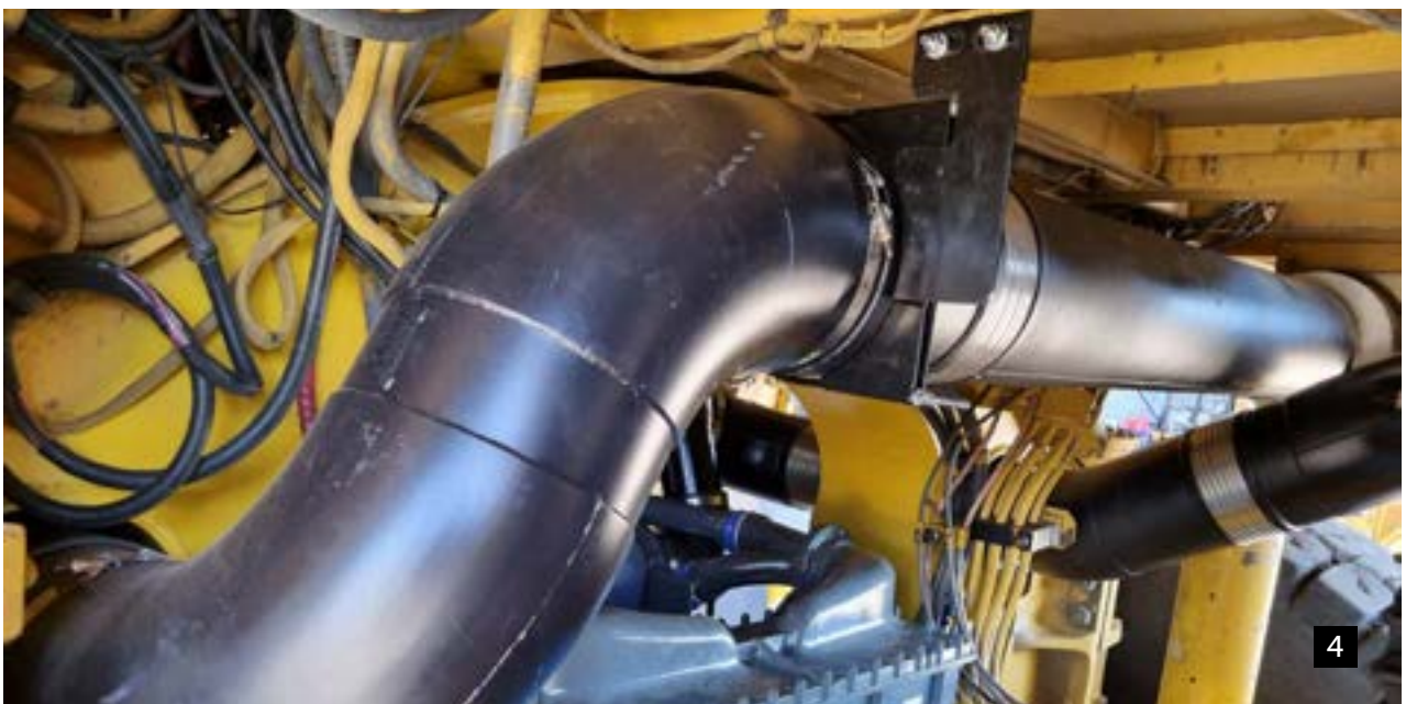
ABOVE Komatsu 830E-AC dual-wall exhaust system, engine pipe and mounting details.
