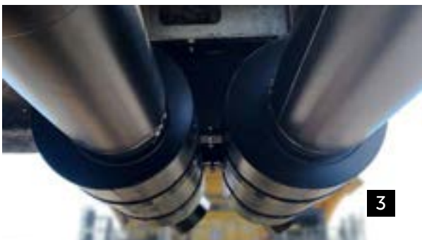
ABOVE Liebherr T282C dual-wall exhaust system, engine pipe and mounting details. Thermal blankets installed on turbos.
