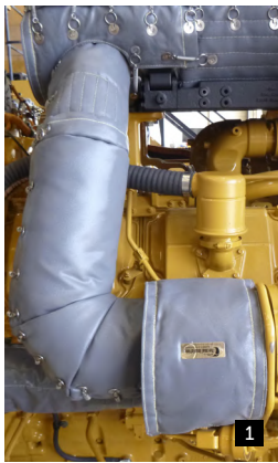
PHOTOS 1-4 Cat D11T manifold, turbo, e/pipe and muffler blankets PHOTOS 5-7 Cat 815K manifold, turbo and e/pipe blankets
