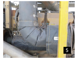
PHOTOS 1-5 Atlas Copco PV275 turbo, engine pipe, muffler and tailpipe blankets. Manifold blankets available (not pictured).
