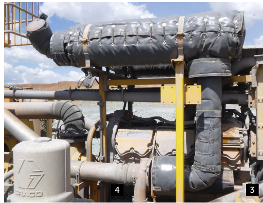
PHOTOS 1-5 Atlas Copco PV275 turbo, engine pipe, muffler and tailpipe blankets. Manifold blankets available (not pictured).
