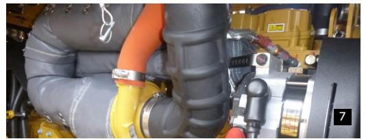
PHOTOS 1-4 Cat D11T manifold, turbo, e/pipe and muffler blankets PHOTOS 5-7 Cat 815K manifold, turbo and e/pipe blankets
