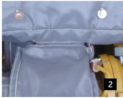
PHOTOS 1-3 Cat 336 manifold, turbo and e/pipe blankets PHOTOS 4-7 Hitachi 5600-6 manifold, turbo, e/pipe and firewall blankets
