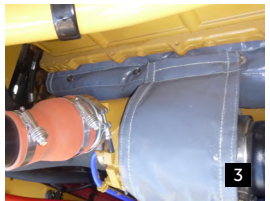
PHOTOS 1-4 PHOTOS 5-7 Cat 24 manifold, turbo, e/pipe, muffler, t/pipe blankets
