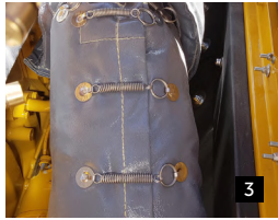
PHOTOS 1-3 Cat 336 manifold, turbo and e/pipe blankets PHOTOS 4-7 Hitachi 5600-6 manifold, turbo, e/pipe and firewall blankets
