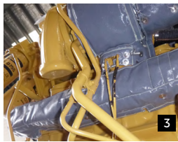
PHOTOS 1-4 Cat D11T manifold, turbo, e/pipe and muffler blankets PHOTOS 5-7 Cat 815K manifold, turbo and e/pipe blankets
