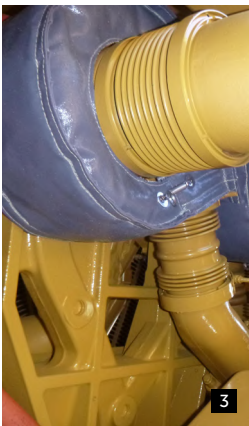
PHOTOS 1-5 Cat 793F manifold, turbo, junction, e/pipe blankets PHOTOS 6-9 Komatsu 830E manifold, turbo, junction, e/pipe blankets
