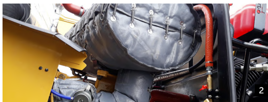
PHOTOS 1-4 Cat 966M turbo, engine pipe, muffler and tailpipe blankets. Manifold blankets available (not pictured).
