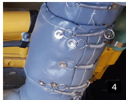
PHOTOS 1-4 PHOTOS 5-7 Cat 24 manifold, turbo, e/pipe, muffler, t/pipe blankets
