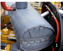
PHOTOS 1-4 Cat 966M turbo, engine pipe, muffler and tailpipe blankets. Manifold blankets available (not pictured).
